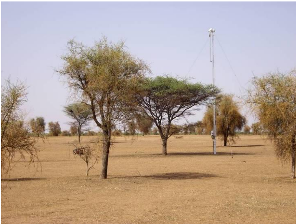
Figure 32: Dahra LST validation station, Senegal. Radiometers observe tree crown, grass and sky BT. Standard meteorology is available from a nearby station of the University of Copenhagen.
