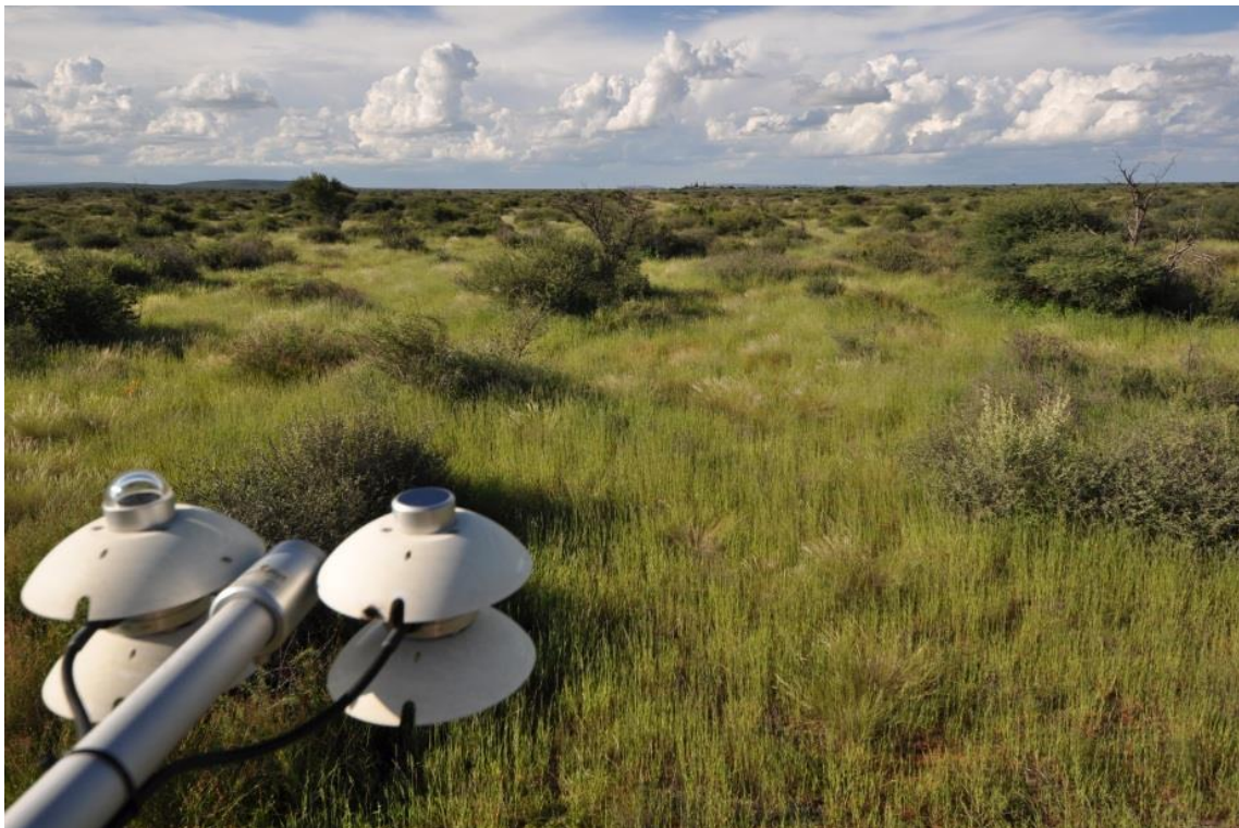
Figure 25: View from mast of ‘Farm Heimat’ LST validation station, Kalahari, Namibia (February 2011; during wet season). In front: radiation balance sensor ‘Hukseflux NR01’.
